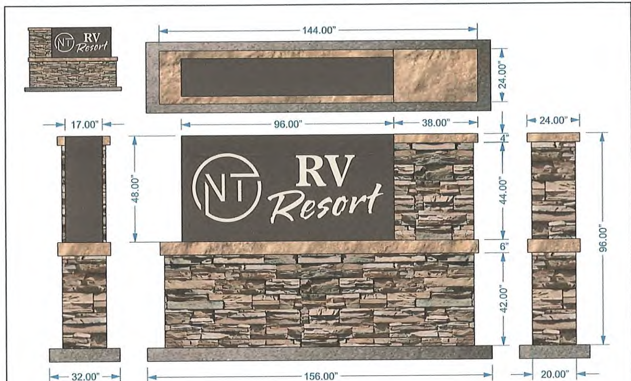
One (1) 96" h x 144" w x 24" d double face illuminated monument sign. The flex faces are 48" h x 96" w. The flex face cabinet is 17" deep.
